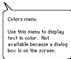
Figure 3-12 A help balloon for a menu title dimmed by the Dialog Manager
